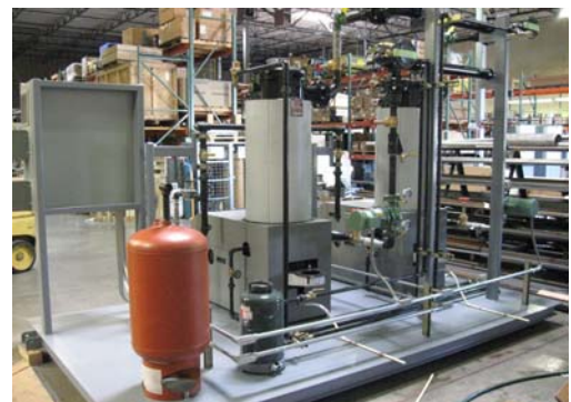
Aerco KC1000 Hot Water Boiler Skid
